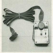
FIG. 7—THE HAND-HELD CONTROLLER allows you to "walk" the mower around the yard to cut a perimeter for it to follow.
